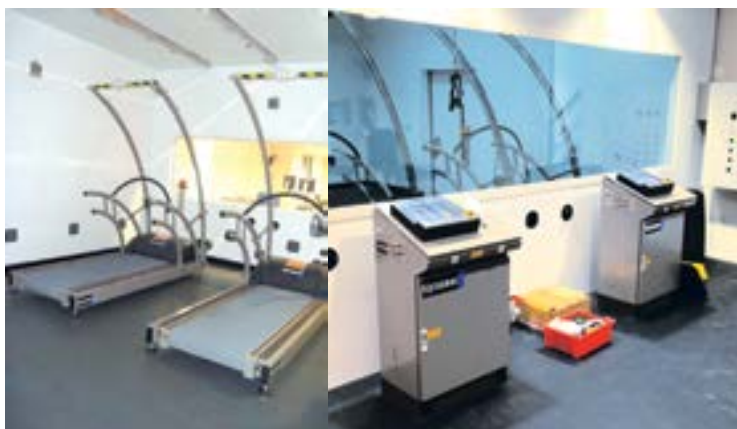
two h/p/cosmos climate-chamber treadmills with external control units outside the chamber for environmental conditions temperature range - 35 ... +50°C (-31 ... +155°F) and humidity up to 100%
