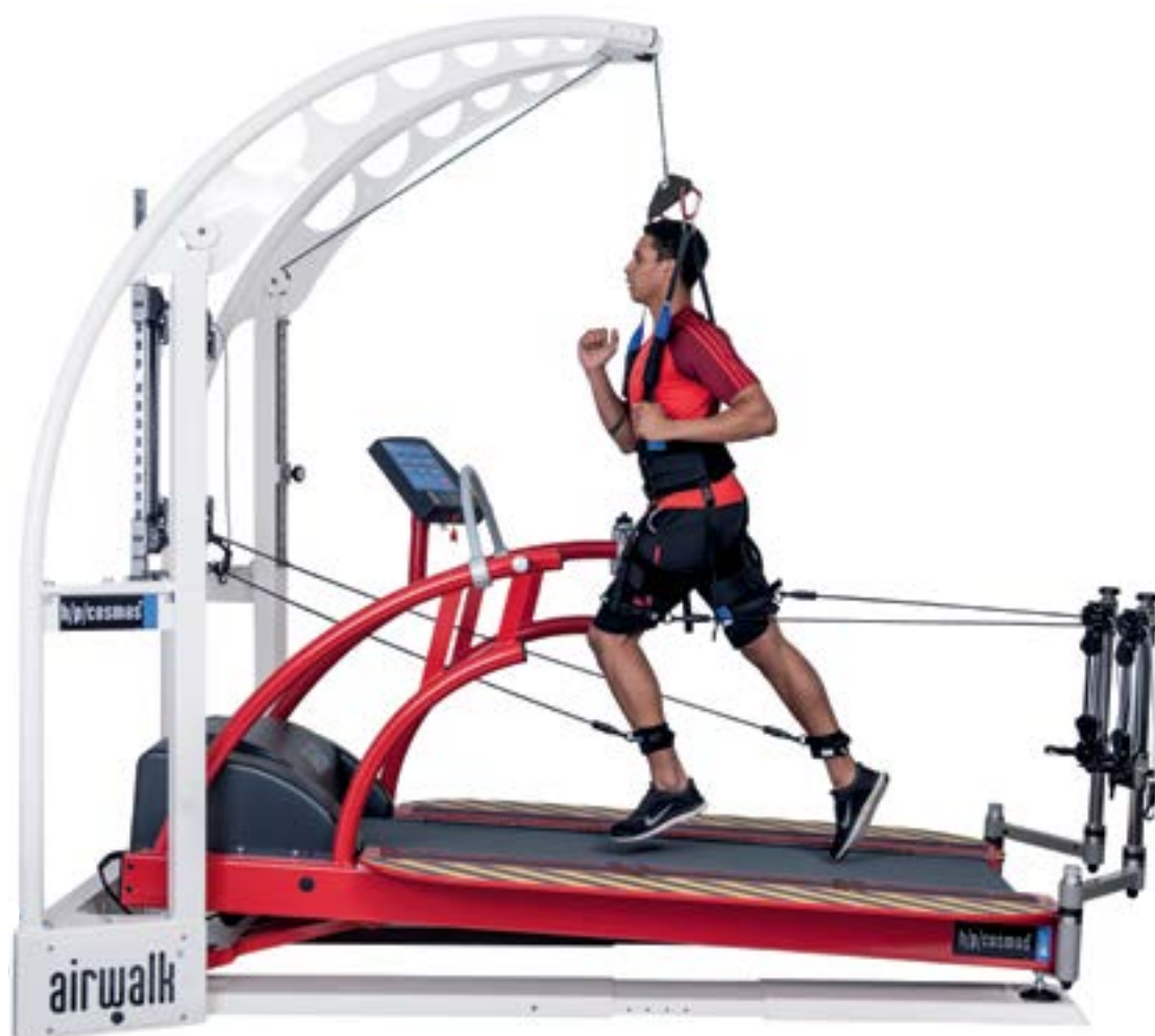
Picture: New h/p/cosmos® system for athletic training, diagnostics and rehabilitation. treadmill pulsar® 3p with overspeed up to 45.0 km/h, speed handrail, extra wide footboards on both sides, robowalk®/roborun® front and back, integrated Microgate Optogait light barrier carpet for step length determination and measurement of biomechanical parameters, pneumatic un-weighting (BWS body weight support) system airwalk® ap with integrated fall stop. The subject is secured against falling and the running belt is stopped automatically in case of a fall.
